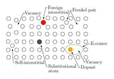
Figure 1: Types of point defects.
